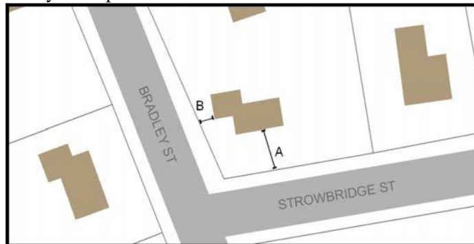
Figure: Corner Lot Yards. The lot shown shall be required to have a full front yard (A) along one street (in the figure, Strowbridge Street) and the front yard (B) along the other street (Bradley Street) at least equal to one-half of the minimum front yard requirements of the district
